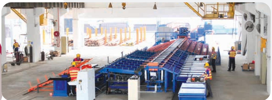
| Automated Cut-and-bend Rebars Processing Plant in Tai Po, Hong Kong
